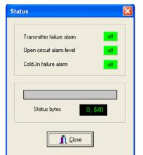
For the two-channel MTL45/5576 the data from channel 1 or channel 2 is selected through the window within the display screen.
