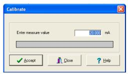
The user must once again read the *measured* loop current on the ammeter, enter the value in place of the 20.00 mA value shown and then click the *Accept* button.
