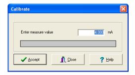
The user is required to read the *measured* loop current on the ammeter, enter the value in place of the 4.00 mA value shown and then click the *Accept* button.
